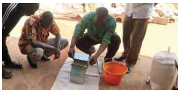
Figure A2 | Example of a “Riffle Divider”
