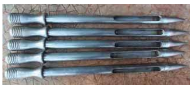
Figure A1 | Example of a “Spear Sampler”
