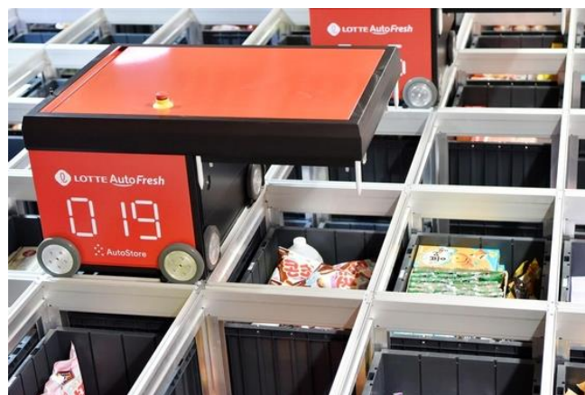
< LOTTE Auto Fresh Center uses total of 19 robots to pick 3,000 items and put them into 7,200 bins allotted for each online order >
